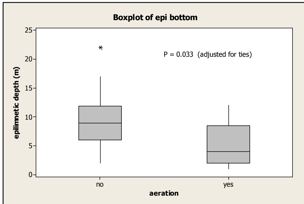
Figure 5 Box Plot of Depth to the Bottom of the Epilimnion During Periods of 'No' Aeration (post-1995) and 'Yes' Aeration (post-1995) for Lake Hefner
