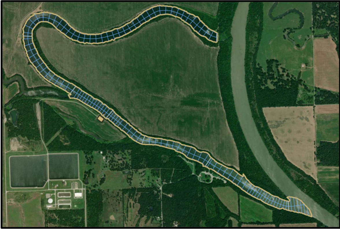
Figure 1. Aerial image of BA Oxbow showing 200 ft transects and centerline for main body with 100 ft transect spacing in areas of concern (intake and inlet/outlet).
