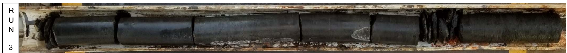
Photo # 3 Run 3 of boring B-5A was from 34.2 to 39.2 feet. Run 3 had a recovery of 93% and an RQD of 78%.
