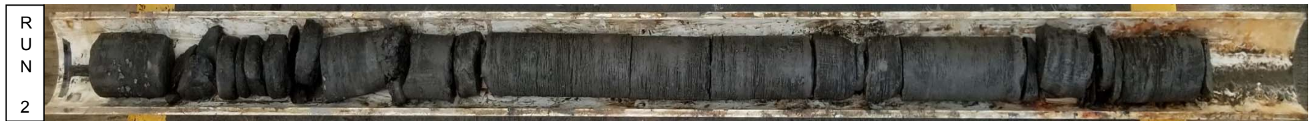
Photo # 2 Run 2 of boring B-5A was from 29.2 to 34.2 feet. Run 2 had a recovery of 91% and an RQD of 28%.
