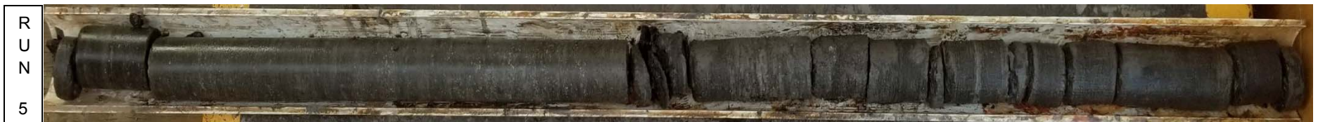
Photo # 5 Run 5 of boring B-5A was from 44.2 to 49.2 feet. Run 5 had a recovery of 97% and an RQD of 55%.
