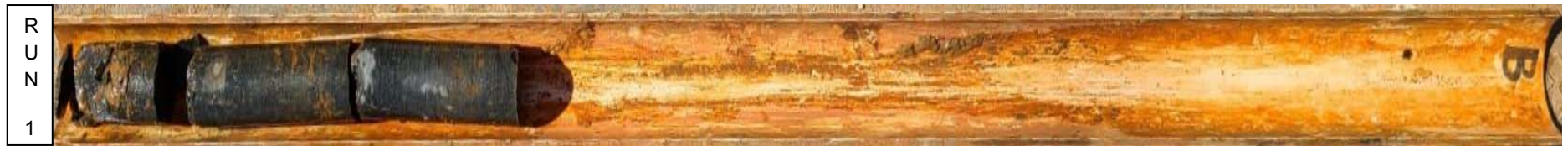
Photo # 1 Run 1 of boring B-8 was from 68.5 to 70 feet. Run 1 had a recovery of 100% and an RQD of 69%.
