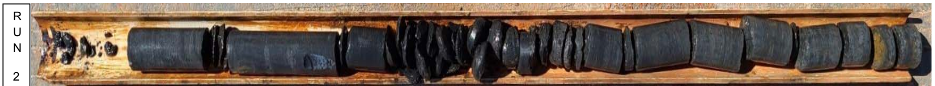
Photo # 2 Run 2 of boring B-8 was from 70 to 75 feet. Run 2 had a recovery of 88% and an RQD of 21%.
