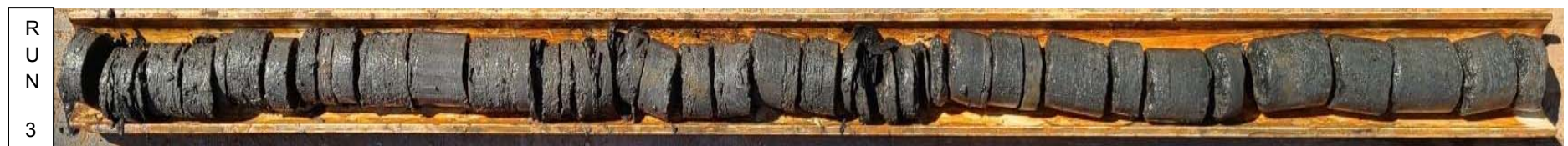
Photo # 3 Run 3 of boring B-8 was from 75 to 80 feet. Run 3 had a recovery of 100% and an RQD of 0%.
