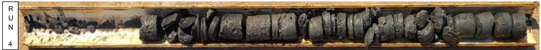
Photo # 4 Run 4 of boring B-8 was from 80 to 85 feet. Run 4 had a recovery of 73% and an RQD of 0%.
