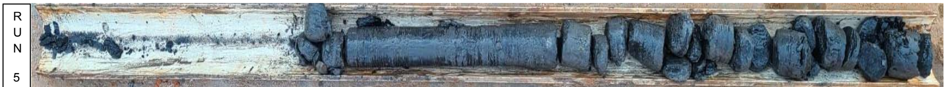
Photo # 5 Run 5 of boring B-8 was from 85 to 90 feet. Run 5 had a recovery of 72% and an RQD of 23%.
