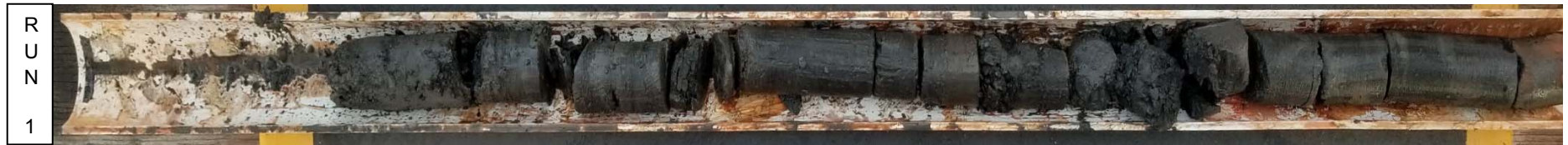
Photo # 1 Run 1 of boring B-5A was from 24.2 to 29.2 feet. Run 1 had a recovery of 82% and an RQD of 23%.
