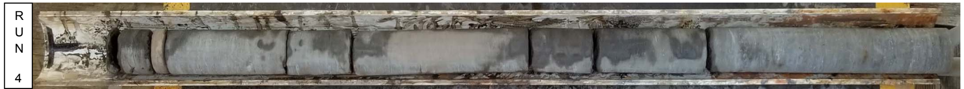
Photo # 4 Run 4 of boring B-5A was from 39.2 to 44.2 feet. Run 4 had a recovery of 93% and an RQD of 83%.
