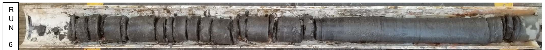
Photo # 6 Run 6 of boring B-5A was from 49.2 to 54.2 feet. Run 6 had a recovery of 90% and an RQD of 33%.
