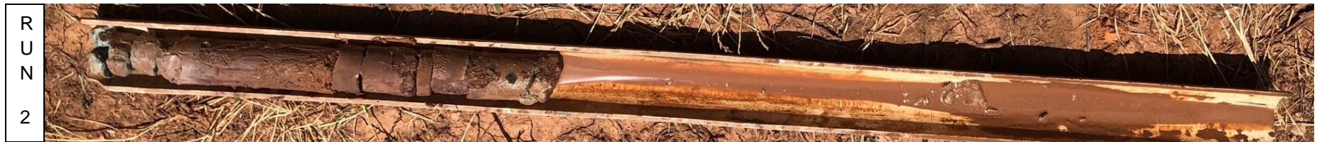
Photo # 2 Run 2 of boring B2-A was from 62 to 67 feet. Run 2 had a recovery of 38% and a RQD of 15%.
