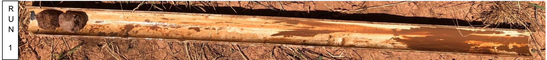
Photo # 1 Run 1 of boring B2-A was from 57 to 62 feet. Run 1 had a recovery of 8% and a RQD 0%.
