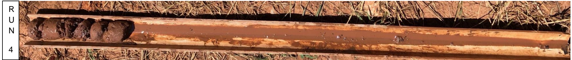
Photo # 4 Run 4 of boring B2-A was from 72 to 77 feet. Run 4 had a recovery of 18% and a RQD of 0%.
