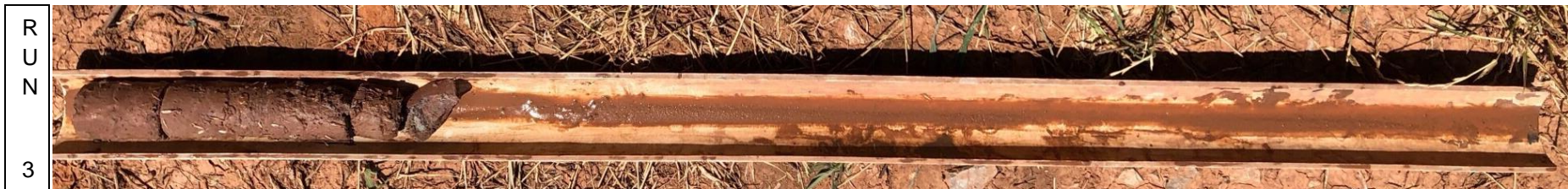
Photo # 3 Run 3 of boring B2-A was from 67 to 72 feet. Run 3 had a recovery of 25% and a RQD of 12%.
