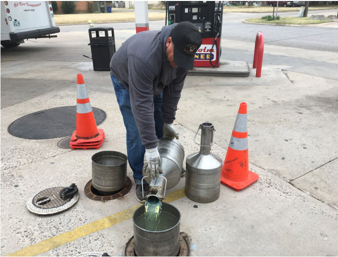
Above: Fuel Inspection Supervisor Ty Massey demonstrates how to return fuel to an underground storage tank after fuel has been tested.
