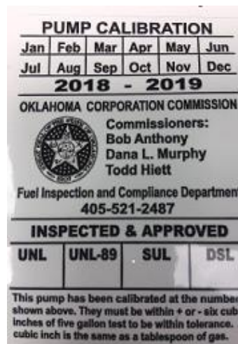
Left: A white calibration label is placed on all dispensers at retail motor fueling facilities indicating the date it was calibrated by a PSTD Fuel Specialist. Inspectors will lock down dispensers not in compliance until the equipment is replaced or repaired to comply with agency standards. The label includes the phone number to report fuel quality issues or any other problems encountered.
