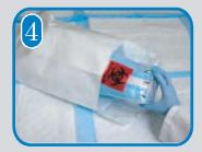
Place the sealed Saf-T-Pak inner leakproof polybag (or equivalent) inside a white Tyvek ® outer envelope (or equilvalent).
