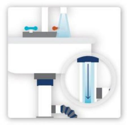
2. After discussing the issue with his supervisor, Jason counteracts the potential for stagnation by daily flushing of the sinks and fixtures with hot and cold water in several rooms including those at the end of the hall, which are farthest from the vertical pipe serving that floor (riser).
