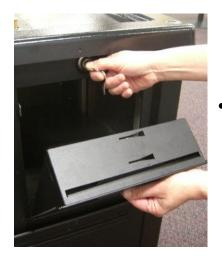
Pull the emergency ballot box door open with the emergency ballot box handle. If it stops after a few inches, continue to pull until it is completely open. Make sure the key latch is in the unlocked position and remove the key from the ballot box.
