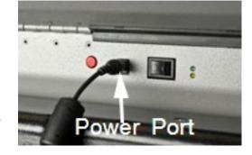
Press the power switch on the back of the eScan to the on position (I). The power lights light up, the eScan start-up screen appears, and an eScan Power Up report prints. Make sure the paper is coming out of the printer and not wrapping around inside. Note: A normal start-up may take three minutes or more, and the console screen may go black for several seconds during the process.
