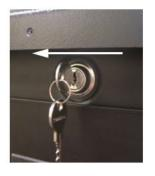
Pull the emergency Ballot box door open with the emergency Ballot box handle. If the door stops after a few inches, continue to pull until it is completely open.
