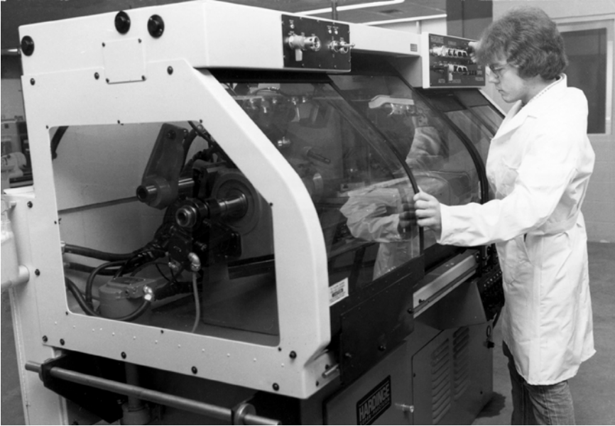
Staying current with advancing technology is a constant challenge for Oklahoma's career and technology education programs. New technology is costly and ages quickly. In this 1990s photo, a student in the machine tool program at Tulsa Technology Center operates an automatic chucker.
