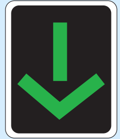
Green Lane open for traffic.
